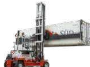
16CS 4H-ECS 7H Tragkraft: 8–9t 4–7 Container stapelbar Antriebsart: Diesel
